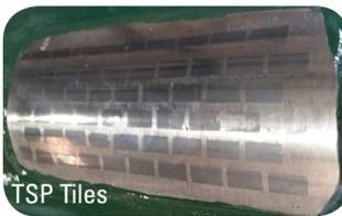
**Carbide Tiles** (Similar to HF 3000) – Amega West holds current “Quick-Tip” certifications in multiple locations. Another variation of Carbide Tiles offered is to use PTA to fill the matrix between the tiles. Advantages include less heat input for non-mag base metal, faster production time, and the addition of carbide particle in the matrix material to reduce wash-out.
