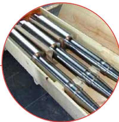
Ring rolling mandrels are finished tooling components that customers can use "out of the box" for hot working operations.
