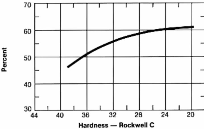
**Core Tensile and Yield Strengths — Carpenter No. 158 Alloy**
