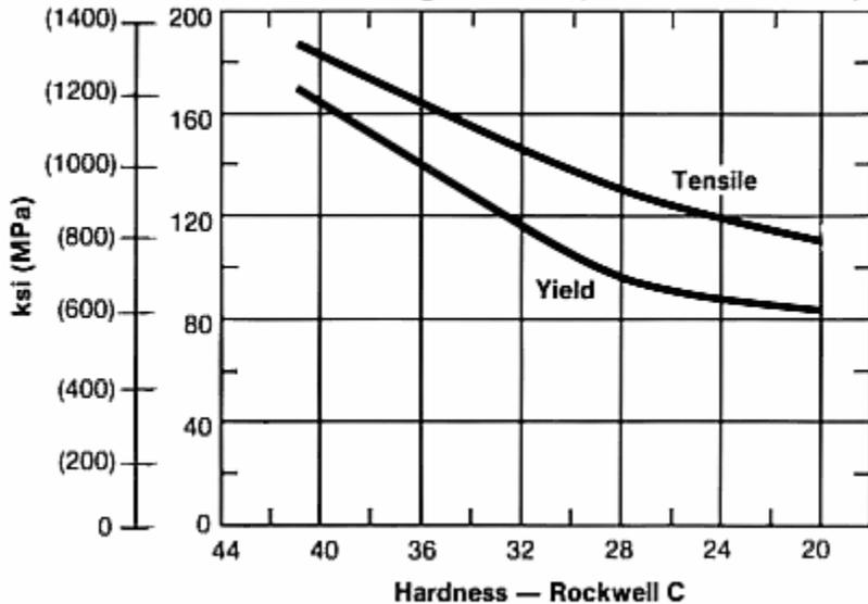
**Typical Case Hardened Mechanical Properties — Carpenter No. 158 Alloy**
