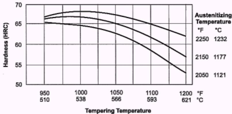
**Effect of Hardening and Tempering Temperatures on Hardness—Micro-Melt T15 Alloy**
