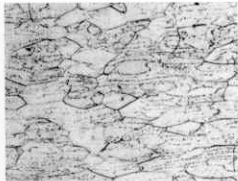
Ti-3-8-6-4-4 Alpha Case in STA Condition
