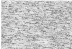
Alpha Case in Ti 6Al-4V
