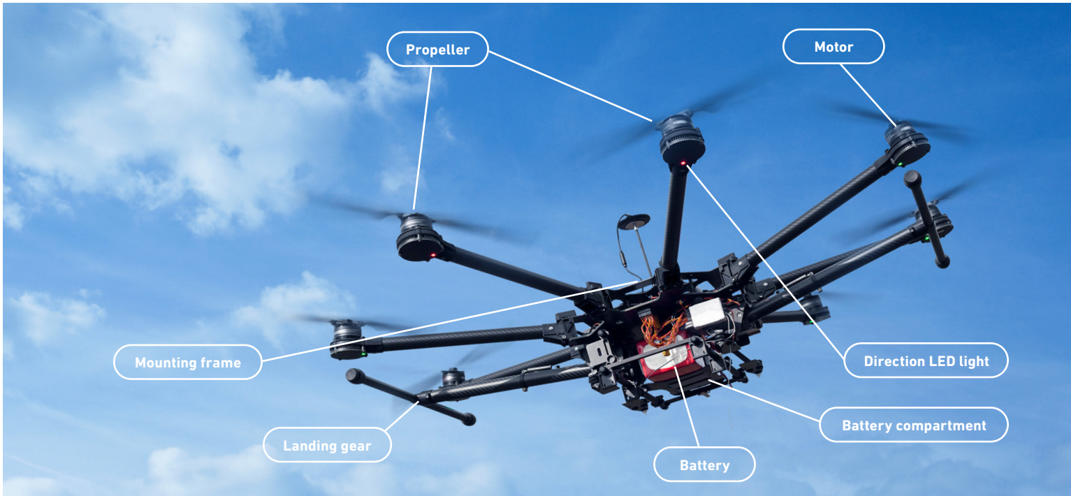
FIGURE 1—HARDWARE COMPONENTS OF A STANDARD UAV
