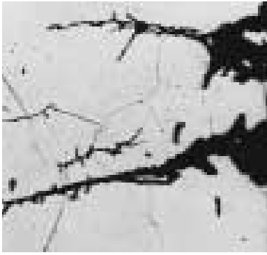
Figure 5: Micrograph of stress-corrosion cracking.
