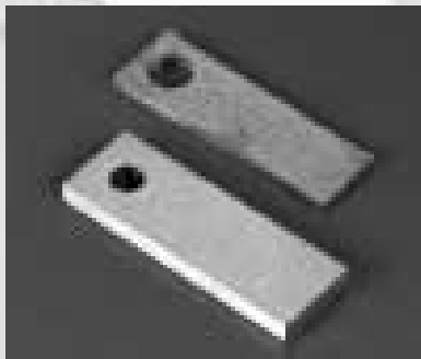
Figure 1: Examples of uncorroded test piece and severe general corrosion.
