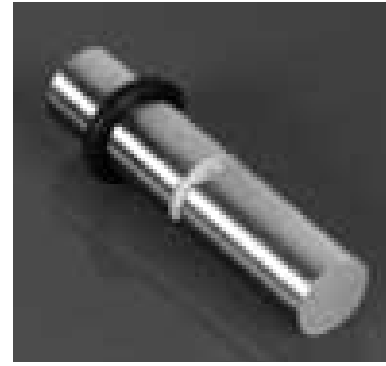
Figure 4: Crevice Corrosion (O-Ring moved)
