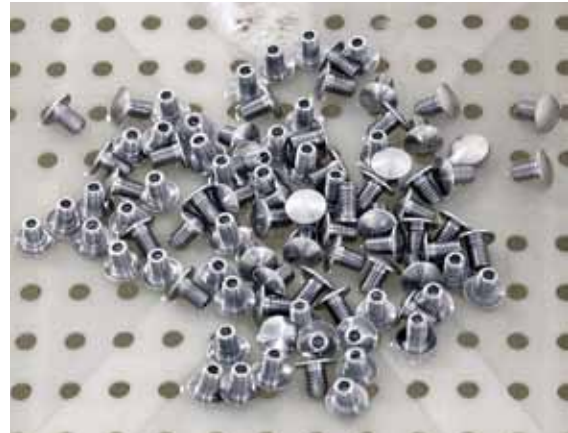
High strength, pin-like surgical instruments made from Carpenter Custom 455® stainless just removed from electropolishing tank. After a deionized water rinse, the instruments will have a lustrous finish. (Photo courtesy of Troy Innovative Instrument, Inc., Middlefield, OH)
