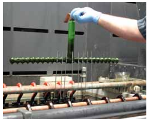
High strength, pin-like surgical instruments made from Carpenter Custom 455® stainless just removed from electropolishing tank. After a deionized water rinse, the instruments will have a lustrous finish. (Photo courtesy of Troy Innovative Instrument, Inc., Middlefield, OH)
