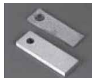
Figure 1 Example of uncorroded test sample and general corrosion
