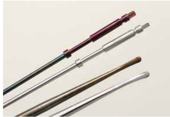
Two small instruments for orthopedic surgery made from Carpenter Custom 455® stainless and Custom 630 stainless. Each bright electropolished instrument contrasts with identical instruments covered by brown oxide from prior heat treatment. Control of finish between bright and dull can be maintained by judicious use of abrasive wheel and fine glass bead blasting. (Photo courtesy of Troy Innovative Instrument, Inc., Middlefield, OH)
