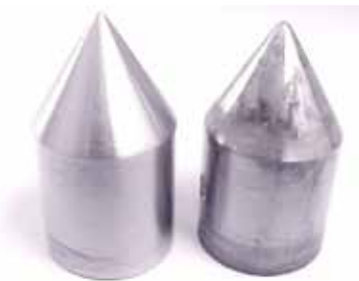
Fig. 1: Left test cone is passivated using the A-A-A method. Results of conventional passivation shown on right. Both were exposed to salt spray.
