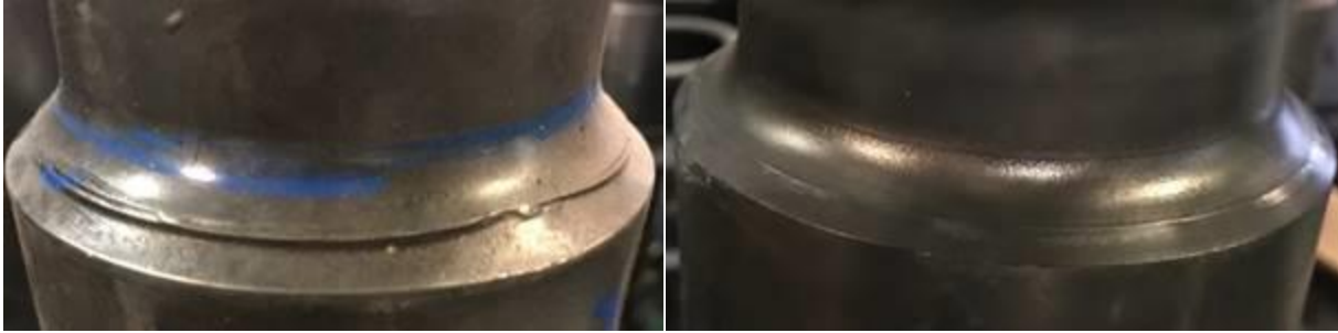
Figure 13: Bearing surface deformation on a 4330+V part (L) is significantly improved with CarTech PremoMax alloy (R).
