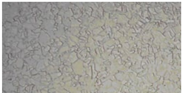
FIGURE 5 — TYPICAL MICROSTRUCTURE OF PM ALLOY 1. WARM WORKED BAR STOCK, LONGITUDINAL SECTION, 1000X, ETCHANT HCL + H 2 O 2 (3%).
